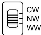
Choose the colour temperature by sliding the switch to the desired position.
